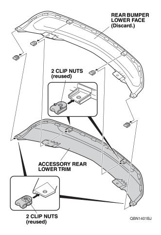
7. Install the rear lower trim to the rear bumper with 4 bolts, 2 clips, and 10 retaining tabs.
